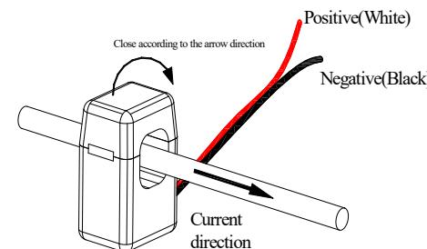
Installation Method of the Open Current Transformer Close
